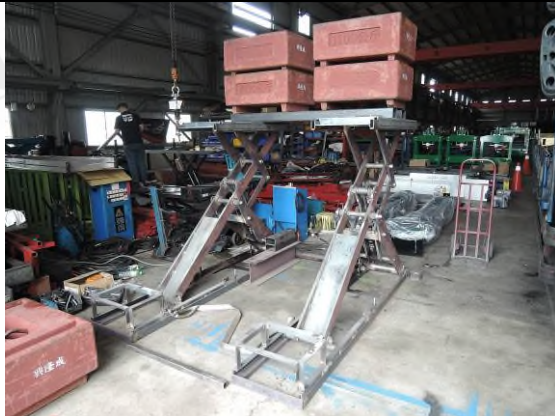
Photo "C" Loading test
