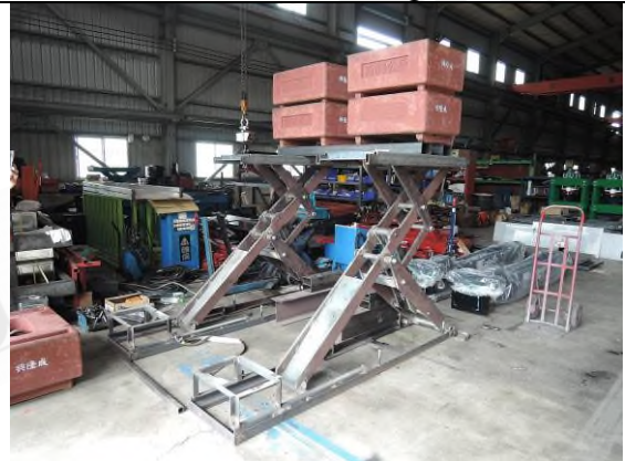
Photo "F" Loading test
