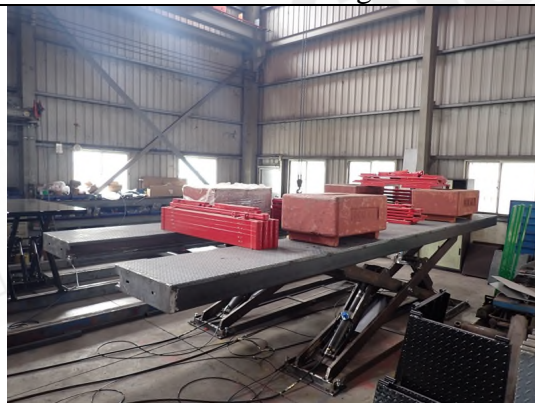
Photo "D" Loading test
