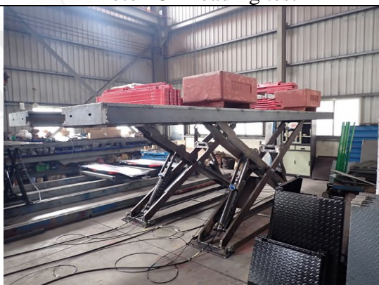
Photo "E" Loading test
