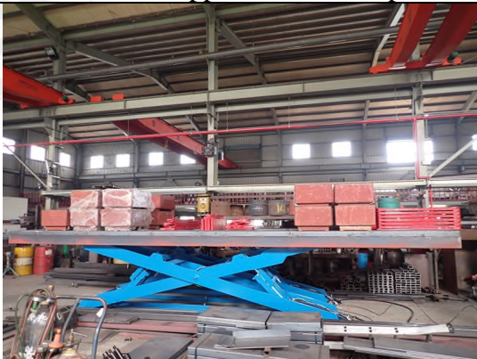
Photo "C" Loading test
