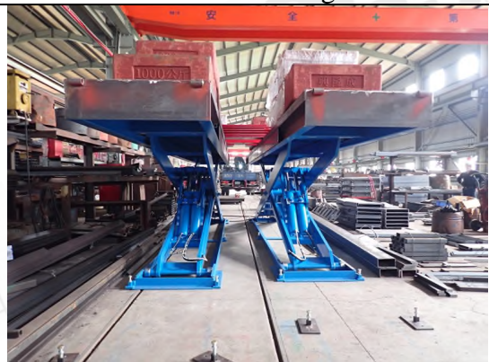
Photo "F" Loading test
