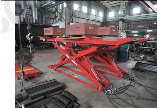
Photo “G” Loading test
