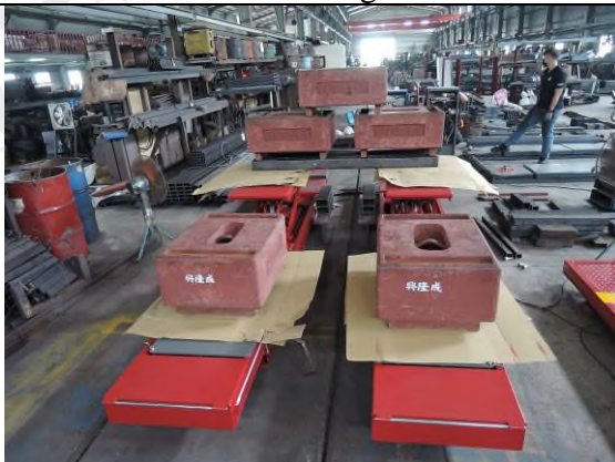
Photo “K” Loading test - 3T
