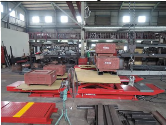
Photo “I” Loading test - 3T
