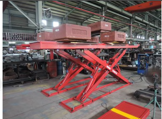
Photo "F" Loading test - 5T
