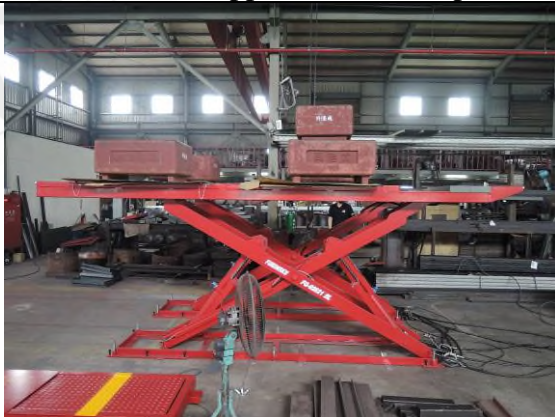
Photo "E" Loading test - 5T
