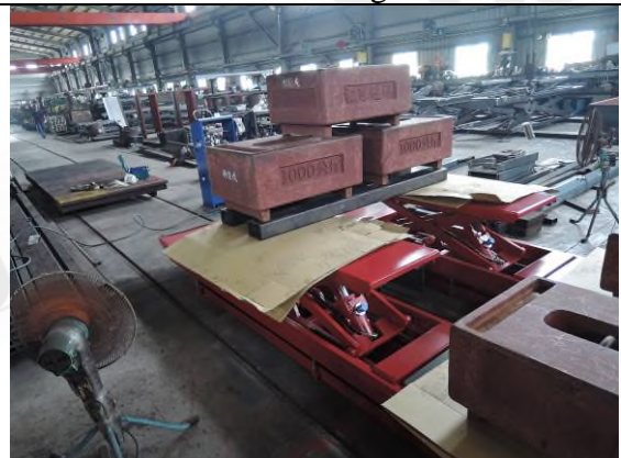
Photo “J” Loading test - 3T
