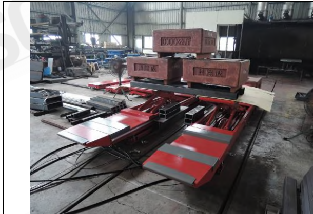
Photo “G” Loading test - 3T
