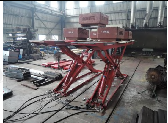
Photo "D" Loading test - 5T
