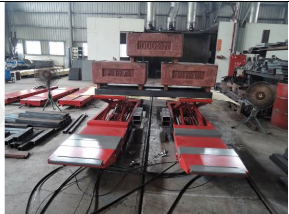
Photo “H” Loading test - 3T
