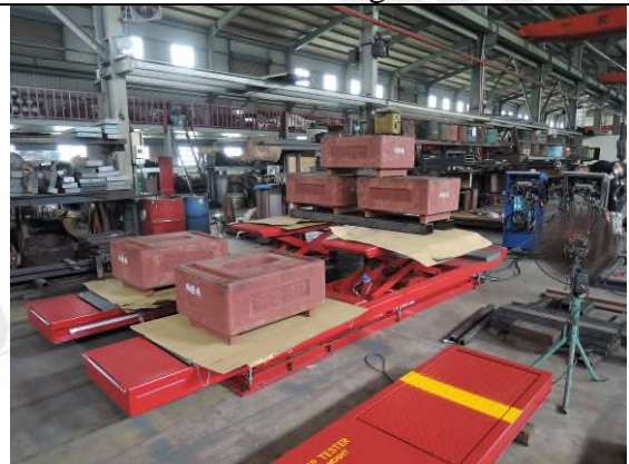
Photo “L” Loading test - 3T
