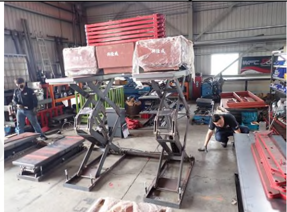
Photo "F" Loading test
