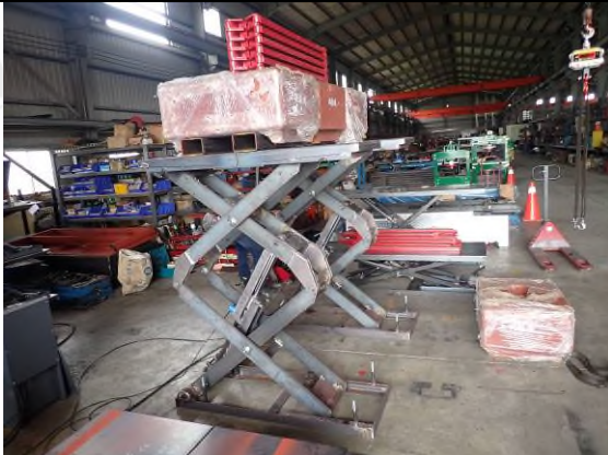
Photo "C" Loading test
