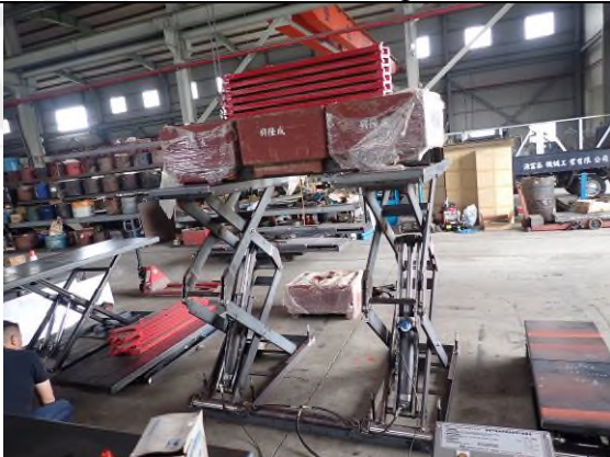
Photo "E" Loading test
