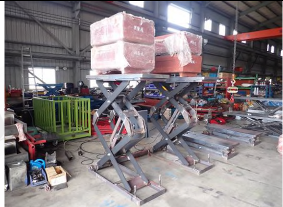
Photo "D" Loading test
