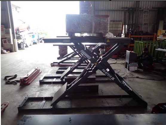
Photo "E" Loading test
