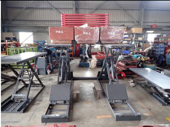
Photo "C" Loading test
