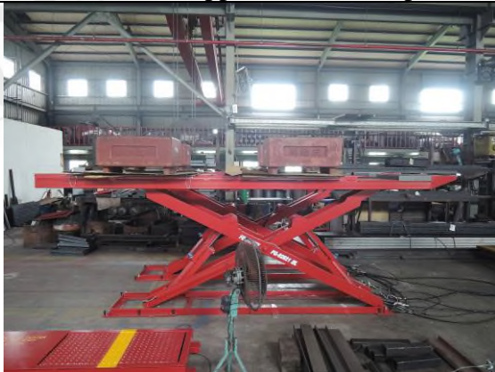
Photo "E" Loading test
