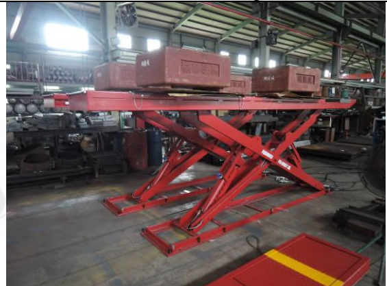
Photo "F" Loading test
