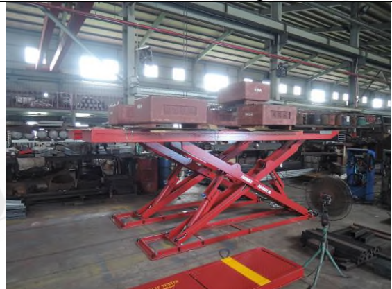
Photo "F" Loading test
