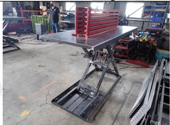
Photo "F" Loading test
